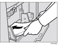
4 Make sure that the paper feed side plates touch the paper lightly. Shift the lock lever backward.
